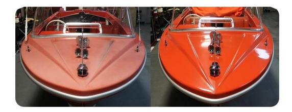
The best medicine for gel coat oxidation is prevention. Follow a simple gel coat maintenance plan to protect your boat's gel coat. If you suspect your boat's gel coat is already oxidized, try these simple tips to remove gel coat oxidation and restore your boat's gel coat to its original lustre.
